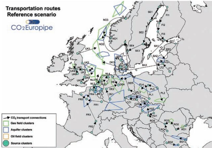
*Illustration of possible future CO<sub>2</sub> transport network: the 2050 reference scenario for CO<sub>2</sub> transport network in Europe, from Neele et al., 2010.*
