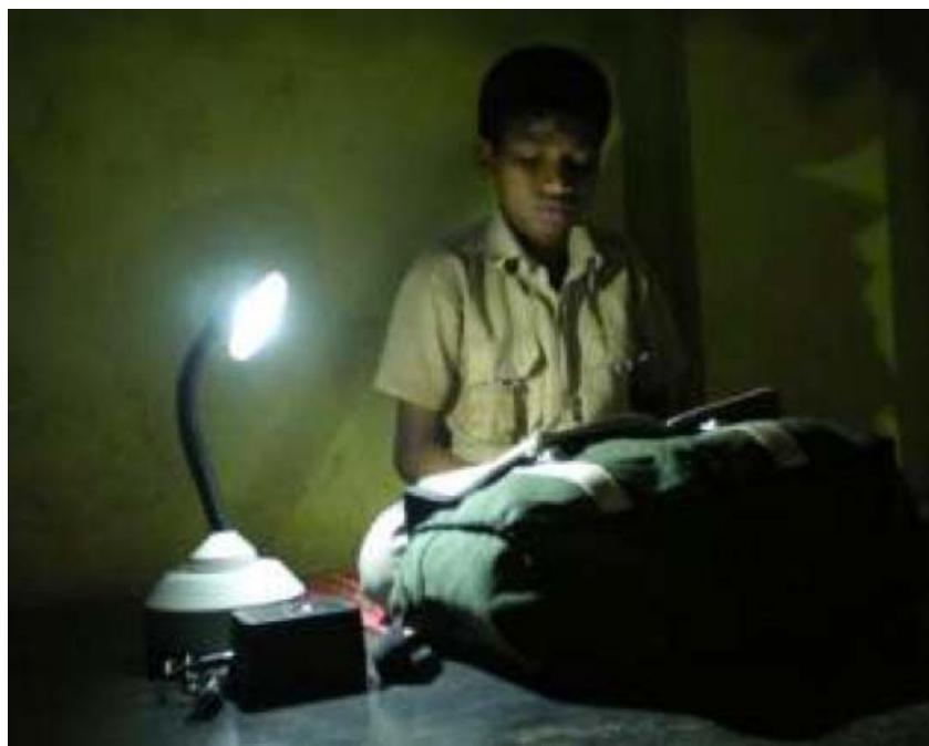
**Figure 4.20: A child studying at night using a hi-power LED study lamp of approximately 0.5W total power consumption. (Source: Selco)**
