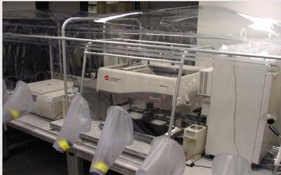
Anaerobic work station in tent
