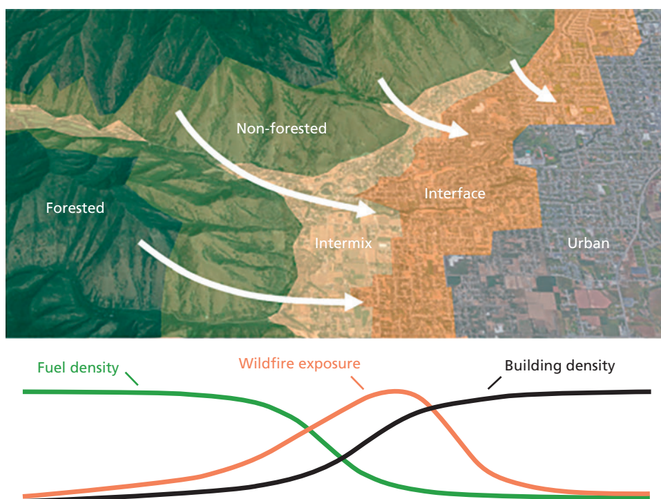
Figure 9 Simplified relationship between fuel density, wildfire exposure, and building density gradients in the WUI (after Ager et al. , 2021).
